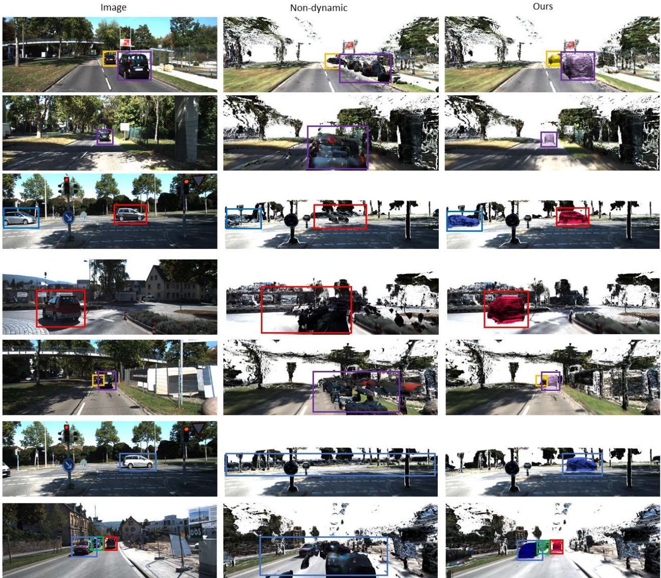
Figure 7. Typical outputs of our system: (left) input images with detected bounding boxes associated over time (trajectories coded by different colours), (middle) Phong-shaded textured output, (right) in our approach, each object is explicitly treated as an independent instance reconstructed in a separate volume; here we visualise it by using colour-coding corresponding to a particular tracklet ID.
