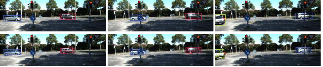
Figure 4. Examples of (dynamic) object detection, data association and 6-DoF object pose estimation. Top: 2D object detection, bottom: corresponding 3D bounding boxes. Note, that colours encode tracklet IDs (data association).
