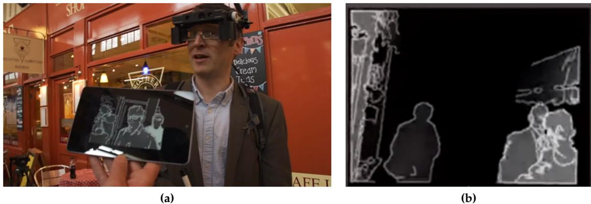
**Figure 4.2:** State-of-the-art technology for helping the visually impaired through AR glasses. This system enhances object boundaries obtained by thresholded depth maps captured by Kinect-like sensors. The depth maps are thresholded in each frame independently and as such are temporary inconsistent and cannot provide the user any semantic knowledge. The use of an active camera limits this system to indoor environments (Hicks *et al.*, 2014).
