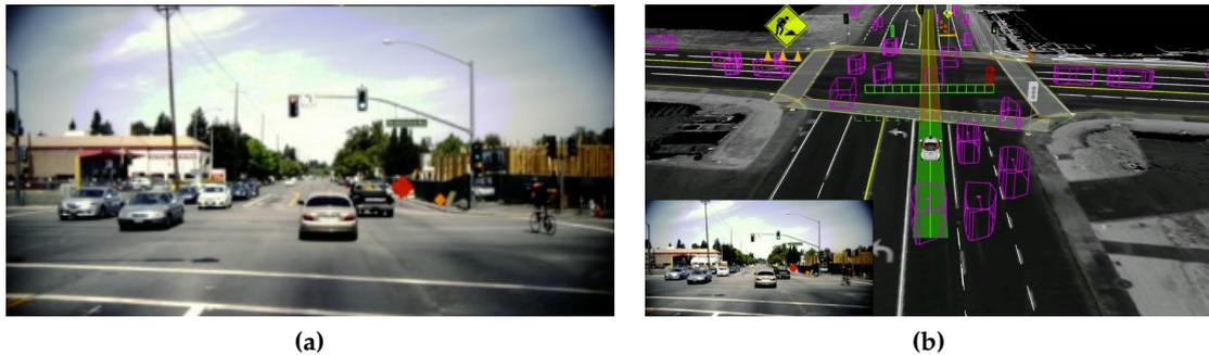
**Figure 1.2:** Google (Waymo) self-driving car relies heavily on intermediate representations. It projects all processed data onto a common metric 3D map to provide situation awareness to the decision making subsystem. This map contains detected and tracked cars, pedestrians, signs and obstacles among others.
