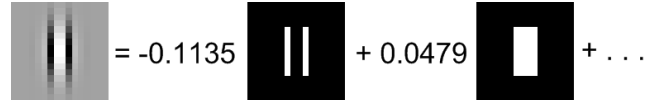
Fig. 1. Decomposition of a Gabor wavelet into a linear combination of Haar-like box functions.
