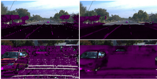
Fig. 4. Learning to predict intensity masks The left column shows real intensity masks from Waymo (top) and SemanticKITTI (bottom) test sets overlaid on the RGB picture. The right column shows the corresponding predictions by RINet.
